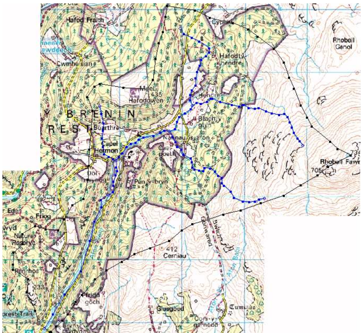
Figure 3.172: Afon Wen MODFLOW model. Base map with boundary and river system defined.
